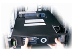
Remove the screws placed on left/right side and extract the unit
